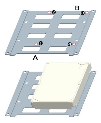
2. Install 2.5" HDD/SSD onto HDD bracket
