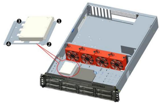
3. Install HDD bracket onto chassis
