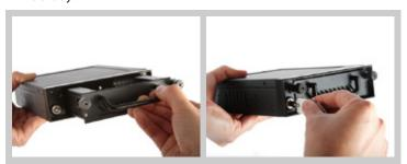
2) Slide HDD into the tray, and make sure the HDD is secured with plastic latch installed.
