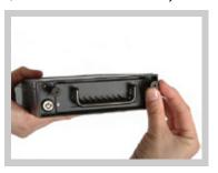
2) Pull the lever outwards and HDD will be release from the backplane as the handle is being pulled.
