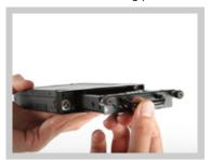
3) Hold down plastic latch and release HDD from the rear (Image 3.1) or unscrew HDD (Image 3.2)
